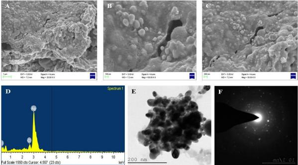
**Fig.2** (A-C) FESEM image of AgNPs at different magnification; (D) EDAX spectrum of AgNPs; (E) HRTEM images of synthesized AgNPs; (F) HRTEM image SAED patterns of AgNPs.
